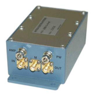
The "AMP" and "PW" controls may be adjusted using a screwdriver.
